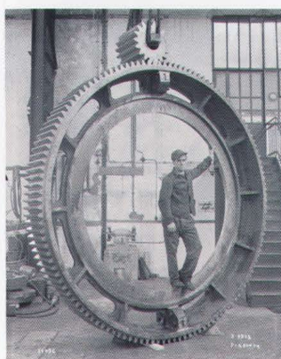
→ Sprocket and large cog, order Z 3973, weight 5,300kg, J. P. Karen (ca. 1950), Institute Emile Metz, CNA Collection.
