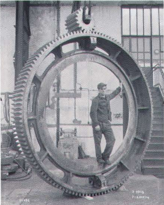
→ Sprocket and large cog, order Z 3973, weight 5,300kg, J. P. Karen (ca. 1950), Institute Emile Metz, CNA Collection.
